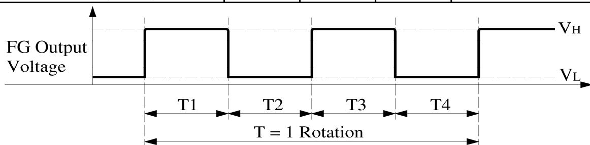
$$T = T_1 + T_2 + T_3 + T_4 = 1 \text{ Rotation}$$
