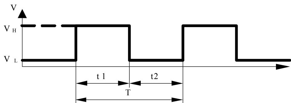
1. Period :  $T = \frac{1}{f_{\text{PWM}}} = t_1 + t_2 (\text{sec})$  .
